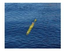
Teledyne Gavia has released a sidescan/bathymetry module that incorporates Klein Marine Systems' UUV-3500 high-resolution sidescan sonar with optional bathymetry sonar. The system is an option for customers interested in utilising the Gavia AUV for geophysical survey, cable and pipeline survey, environmental survey or under-ice survey, as well as mine countermeasures (MCM), rapid environmental assessment (REA), or intelligence, surveillance and reconnaissance (ISR) surveys.
