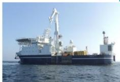
A new Kongsberg EM2040D has been installed on MMT's long-term charted multipurpose support vessel Stril Explorer. The device has a 0.4 x 0.7 degree dual-head multibeam system and it combines all of the features of deepwater echosounders for the shallow-water or ROV/AUV environment.
