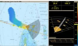
FarSounder has announced its Local History Mapping (LHM) feature, which offers users the ability to build a 3D map of the seafloor over which they have recently sailed. This map is updated with every ping and is displayed as an overlay on top of the system's nautical chart display. This new overlay is displayed in conjunction with the real-time sonar overlay. This combination enables users
