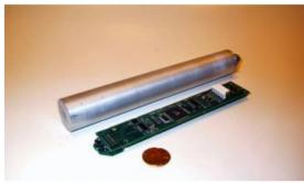
AOSI's newest EZ-Compass-3AL Logging Compass incorporates a three-axis magnetometer with tilt and temperature compensation and a high capacity integrated logger that allows independent storage of up to 20,000 measurements, which are easily transferable to any PC. The 1.5" x 2.0"x 0.5" module weights about 11gr and outputs heading, pitch, roll, magnetic field and temperature over RS232 and RS422/RS485 ports by using all solid state components.
