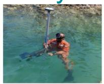
A two-person Astrolabe Engineering survey team using a single SP60 GNSS receiver recently completed the entire land and sea route for the world's longest and deepest alternating current (AC) cable.
