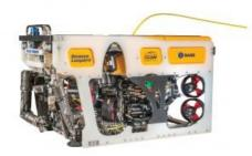
Specialist submarine cable installation company Louis Dreyfus TravOcean, France, has ordered two Saab Seaeye Leopards for touchdown monitoring and support. The pioneering Leopard work vehicle, with its 11 thrusters and iCON intelligent control system, will provide TravOcean with a stable work platform that is unrivalled amongst ROVs – particularly in strong currents.
