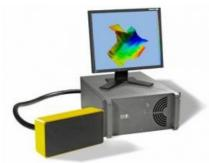
A new cost-efficient sonar bridging the gap between singlebeam echosounders and high-resolution multibeam sonar systems is the HydroBat, a multibeam system operating at 160kHz and covers a swath of 120Ű. Rich Lear at RESON explains the significance: "A task that used to take a week with the old singlebeam echosounders, takes only three days with this new multibeam HydroBat."
