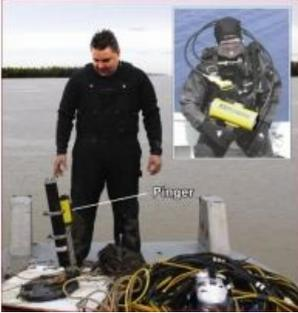
JW Fishers, USA, has recently added a new low-frequency pinger to its line of acoustic devices. The new model has a significantly longer transmission range (3 to 6 miles compared to 2,000-3,000 feet for a conventional pinger), a longer battery life, and a variety of other new features including delayed start which allows the pinger to lie dormant for up to a year before beginning to transmit.
