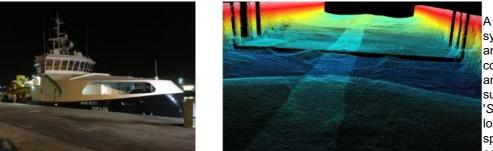
A complete multibeam echosounder system and high-speed winch designed and engineered for optimal durability compose the scope supplied, installed and set to work by MacArtney's French subsidiary. The newly built rescue vessel 'Sirius', operated by VLOOT dab, is 45m long, almost 11m wide and can reach a speed of 13 knots. Being intended for combating disasters at sea, 'Sirius' was
