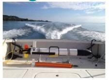
OceanServer Technology, USA, has partnered with Marine Magnetics to bring a new magnetometer option to the Iver2 family of AUVs. This new AUV-towed device, coupled to enhanced data-logging software features, enables existing or new Iver2 AUVs to collect high-quality georeferenced magnetometer data.
