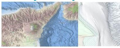
The EMODnet DTM with digital bathymetry for all European waters has again been updated in the last year and is now publicly available for browsing and downloading from the portal. The number of survey datasets and composite DTMs used as data sources has increased from approx. 7,000 to more than 7,700. These survey datasets have been contributed by 31 data providers from 18 countries and
