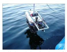
In recent trials off Trondheim, Norway, the GeoSwath Plus swath bathymetry and side scan system was used for the first time on a remotely operated vehicle (ROV) to map cold water coral reefs. The objective of the survey was to test how effective the GeoSwath was as a ROV mounted sonar for identifying cold-water coral colonies.
