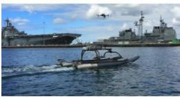
Marine Advanced Robotics and Planck Aerosystems have established a strategic alliance to provide a multi-domain robotic team that includes an unmanned surface vessel (USV) equipped with a small unmanned aircraft system (sUAS) that operate together for advanced mission profiles.
