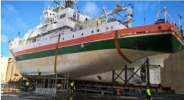
The almost-30-year-old 'Aranda' will undergo a renovation at the Rauma Marine Constructions (RMC) shipyard in Rauma, Finland. The modifications will involve a sevenmetre extension to the vessel, which will become more environmentally friendly. The refurbishment of the research vessel requires special expertise, which in the best-case scenario may result in more work for Finland.
