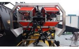
vehicle has been installed on board the shadow boat *HODOR* as the rescue unit for the *SEAmagine Aurora* 3 manned submarine, which this vessel carries and operates. Like the *Aurora*, this ROV has a working depth of 1,000 metres, thus guaranteeing support throughout the whole depth range in which the submarine operates.
