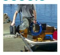
Teledyne Odom Hydrographic, USA, has announced the launch of the MB2, the first product since the MB1 introduction in 2012. The MB2 multibeam echosounder is developed for fast mobilisation on smaller vessels and is optimised for shallow-water survey companies, port and harbour authorities, dredging companies and other users looking for an easy-to-use, quick-to-deploy, high-resolution system.
