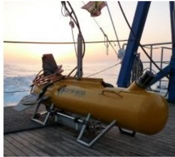
The Applied Acoustics deep-tow sparker, the DTS-500, has recently been deployed in the Mediterranean Sea, off the continental slope of Majorca, working on a project with SOCIB, the Balearic Islands coastal observing and forecasting body. Assisted by Carlos Castilla Álvarez, SOCIB's oceanographic instrumentation technician, the DTS-500 was deployed in deep water, up to 500m, at a distance up
