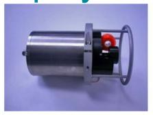
The MINIpack CTD Fluorimeter has been optimised for use in the Antarctic. The MINIpack is a very compact sensor and it has now been complimented with a low-profile guard specifically designed for deployments through ice holes. A standard ice auger hole is 250mm diameter. With the new guard the MINIpack diameter only increases from 120mm to 140mm making it suited for measurements through ice boreholes.
