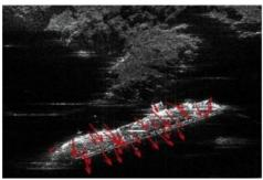
TRE and the Polytechnic University of Milan, Italy, in collaboration with the Department of Earth Sciences (University of Florence) have been monitoring the movement of the partially submerged cruise ship Costa Concordia since 20th January 2012 off the coast of Giglio Island. High-resolution images from the Italian COSMO-SkyMed constellation of satellites are being used to provide information on the position and movement of the ship, for integration with ground warning systems.
