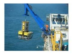
UK-based Bibby Offshore have taken delivery of two SMD Quantum MkIII 250hp 3,000m rated Work Class ROVs, increasing their ROV fleet to nine SMD vehicles - including one Atom and six Quasars. Each of the high specification Quantum Work Class ROV systems includes SMD's Extended Tophat Tether Management System (TMS), telescopic A-Frame, umbilical winch, deck pack and fully integrated control cabin.
