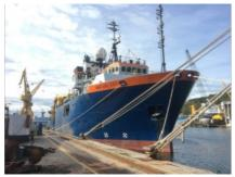
Lighthouse continues to invest in enhancing the capabilities of its survey fleet, with the recent arrival of the MPV/DP2 'Nautical Geo', Lighthouse's latest multipurpose offshore vessel. 'Nautical Geo' is a 74m-long, DP2-class research vessel, fitted with payload capable to cover a wide range of services.
