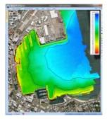
Chesapeake Technology (Canada) has added post-processing for multibeam echosounder and interferometric bathymetry systems to the SonarWiz software. SonarWiz now offers data processing for bathymetry file types of ALL, HSX, JSF, R2S, RDF, S7K, SXI, and XTF. SonarWiz Bathy reads the native data formats directly and gives the user all the tools required to view and edit the bathymetric data to produce high-resolution maps and reports.
