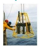
OSIL's range of Bowers and Connelly Multiple Corers are capable of collecting an undisturbed sediment sample from the seabed. Each of the four corers, Mega, Maxi, Midi and Mini use a hydrostatically damped coring mechanism to attain the undisturbed sample.
