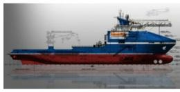
SENER, Spain, is developing a multipurpose subsea support vessel especially designed for subsea ROV (remoted-operated vehicle) light construction duties, for worldwide service. The ship will have a length overall of more than 112m, a length between perpendiculars longer than 100m and a breadth of 22m. The depth to main deck will be 9m while the draft will have more than 7m. In total, it will be able to accommodate 110 persons on board.
