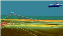
NaviCat software is able to execute catenary simulations related to anchor handling tug operations through integration with EIVA NaviPac including 3D visualisation option. By utilising predefined cable, MLB and anchor libraries NaviCat makes creation, modification and display of catenaries extremely easy and intuitive.
