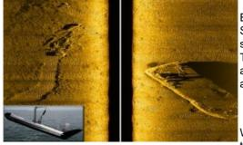
EdgeTech, USA, recently added a new frequency pair to the popular 4200 Sidescan Sonar. The EdgeTech 4200, a multi-purpose survey system that can be configured for shallow or deepwater operations, is now available with a 100/600kHz frequency pairing. This dual simultaneous frequency combination gives surveyors the ability to achieve an along-track resolution of 2.5 metres at 200 metres range (with MP Technology) and 0.45m at 100 metres range. Across-track resolution is 8cm and 1.5cm respectively.
