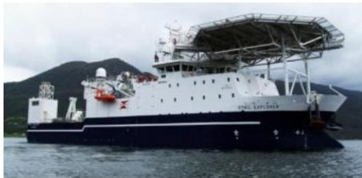
As a natural next step in the process of expanded subsea services in the oil and gas industry, MMT has signed a long-term charter contract for M/V *Stril Explorer* that is operated by Simon MÅkster Shipping AS. *Stril Explorer* has one main ROV hangar, suitable for 2 x WROV, launching through hangar port/starboard side doors. The vessel is also equipped with a separate deck hangar suitable for 1 x IROV launching through a side door.
