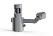
Newton Labs' M series of underwater laser scanners can be utilised for area scans or as a fixed-line scanner coupled to an IMU/DVL for long-distance scans such as pipelines and umbilicals, etc. The same scanner can be used for high-resolution area scans and dynamic field scans at the push of a button on the user interface.
