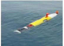
Autonomous underwater vehicles (AUVs) can perform subsea cable surveys faster and more economically than ships with towed instruments, according to a recent study of researchers from the Woods Hole Oceanographic Institution (WHOI). "AUVs can cut down on ship costs and weather delays while reducing the time required to gather the data operators need to assess their underwater infrastructure", said Anthony Kirincich, a physical oceanographer at WHOI.
