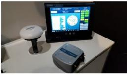
Oceaneering has announced the release of the C-Nav5000 GNSS receiver, which uses 252 tracking channels capable of tracking phase and code of all available constellations, including GPS, GLONASS, Beidou and Galileo.
