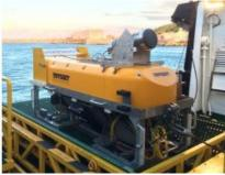
Odyssey Marine Exploration has successfully evaluated subsea technology allowing a geophysical towfish to be tracked at distances far greater than current methods allow by during trials in the Bay of Biscay. The Sonardyne Ranger 2 GyroiUSBL system was able to track Odyssey's latest deep tow side-scan platform at a slant range of 7,500 metres from its vessel, *Odyssey Explorer*. Only the depth of the ocean prevented greater ranges being achieved.
