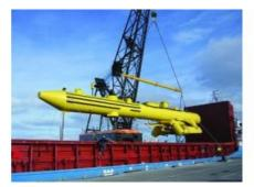
In the summer of 2011, Orkney-based Scotrenewables launched its prototype floating tidal turbine, the SR250, designed to minimise the installation and maintenance costs of tidal energy compared to seabed-mounted tidal turbines.
