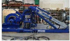
Okeanus Science & Technology has delivered a self-contained, rapid-mobilisation remotely operated vehicle (ROV) launch & recovery system to Phoenix International in Largo, Maryland, USA. The fully integrated system, designed and built to launch and recover a free-flying ROV, contains a winch/level wind assembly, self-erecting A-Frame, docking head/over-boarding sheave assembly and electro-hydraulic power unit, all mounted to a single skid.
