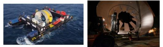
It is crucial for tidal turbine manufacturer OpenHydro to obtain precise current, wave and turbulence information as it is delivering two of the world's first grid connected tidal arrays. OpenHydro has opted for the <u>Nortek Signature500 current</u> <u>profiler</u> to optimise the operational speed of these 16-metre-diameter devices. Two such turbines have already been deployed on EDF's Paimpol-Bréhat project in
