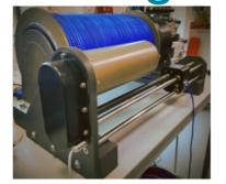
The marine engineering experts from Ocean Scientific International (OSIL) have produced an innovative and compact autonomous profiling winch that will operate unmanned for 30 days. OSIL were approached with a requirement for a 24V waterproof winch system to mount to existing Automated Surface Vehicle system. The winch will undertake ten profiles per day, with a 15kg payload, for 30 days continuously.
