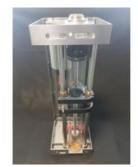
UK-based Ocean Scientific International (OSIL) has announced the release of an innovative new sediment corer designed to be mounted to the skids of ROVs or AUVs. The self-contained system will allow sediment samples to be collected during routine ROV operations and can be daisy chained together to allow multiple core assemblies to be installed as one system.
