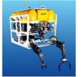
Saab Seaeye has launched the Panther XT, a more powerful, deeper swimming version of their successful Panther Plus ROV with a much greater tooling capability. It comes as world sales of the Panther range of electric work-class ROVs exceed 30 vehicles. ROV operators will benefit from technology that has doubled thruster power and increased performance. This comes through increased thruster motor voltage from 250V to 500V.
