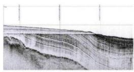
Knudsen Engineering have put their new 15kHz Pinger sub-bottom profiling system through its paces on Lake Champlain Vermont with the support of Middlebury College on their research vessel R/V Baldwin. During the demonstration the Pinger was operated in water as shallow as 1.5 metres. Shallow water has always been a problem for conventional SBP's because of transmission pulse ringing. Data processing was performed with Chesapeake Technologies SonarWiz 5 software.
