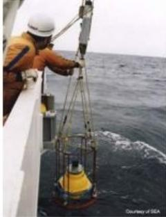
LinkQuest's Precision Marine Geodetic Systems (PMGS) are specially designed for seafloor movement monitoring. They are capable of accurate positioning within 0.5cm for up to 7,000m in range. LinkQuest has been working with the Japan Marine Safety Agency (JMSA) and Japan Coast Guard since November 1999, and more than 100 PMGS transponders have been deployed on Japan's sea floors.
