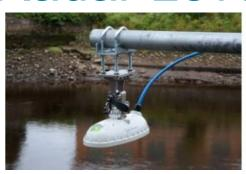
The Valeport VRS20 Radar Level Sensor uses non-contact technology and can be installed easily. The device uses 25GHz pulsed k-band radar to measure water level to an accuracy of ±10mm. It has been designed to work with Valeport's TideMaster tide logger or to operate as a stand-alone device with optional integrated GPRS telemetry. Alternatively it can interface with a third-party data logger.
