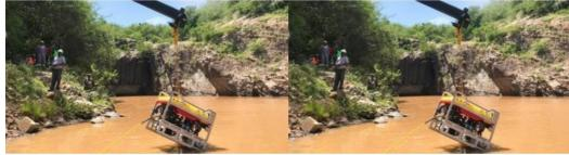
ASI Group, a global specialist in inland waters, has deployed a Saab Seaeye Falcon robot into crocodile-infested waters in East Africa to inspect and survey the infrastructure supporting five power stations. The crocodiles had been preventing the manual inspection of remote inland underwater structures.
