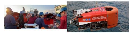
A hybrid remotely operated vehicle took the first known automated sample performed by a robotic arm in the seabed of the Greek island of Santorini. The vehicle, developed by Woods Hole Oceanographic Institution (WHOI), explored Kolumbo volcano, an active submarine volcano off the famed island.
