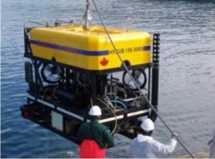
ISE has delivered a new Remotely Operated Vehicle (ROV) for SNK Ocean Co. Ltd., a Japanese marine services company based out of Tokyo, Japan. SNK has other ISE equipment. The HYSUB ROV, the 'Hakuyo 150-3000', is designed to perform functions including cable burial, salvage, research and survey. It is SNK's deepest-diving ROV, rated to an operational depth of 3,000 metres.
