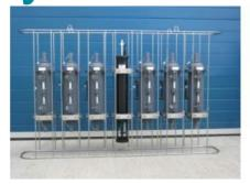
OSIL have supplied a water sampling system of for use in the offshore oil industry. Iindustry-standard Niskin bottles are included due to their robustness. OSIL designed a sampling system to secure 6 primed 5L Niskin bottles, with space for an AML Oceanographic CTD Plus V2 in the centre of a stainless steel frame, which could then be mounted to the ROV.
