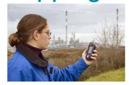
Magellan has introduced the latest addition to its MobileMapper GIS and mapping line of products - the MobileMapper 6. A rugged, waterproof, handheld GPS/GIS receiver, the MobileMapper 6 fulfills the requirements for low-cost, professional GIS field data collection.
