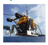
For pipeline inspection in the Gulf of Mexico, global maritime, survey and ROV services operator ACSM chose an electric Saab Seaeye Panther XT robotic vehicle over other ROV vehicle alternatives.
