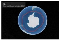
A seven-meter (23-foot) long, wind-powered unmanned surface vehicle (USV), called a <u>saildrone</u>, has become the first unmanned system to circumnavigate Antarctica. The vehicle, known as SD 1020, was equipped with a suite of climate-grade sensors and collected data in previously unchartered waters, enabling new key insights into ocean and climate processes. The SD 1020 survived
