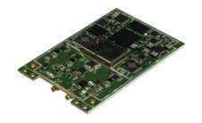
SBG Systems has selected the Septentrio AsteRx4 OEM GNSS receiver to equip the Apogee product line. The Apogee is a new product line of highly accurate inertial navigation systems based on robust and cost-effective MEMS technology. The INS/GNSS solution combines the latest generation of MEMS sensors and the OEM version of the AsteRx4, a newly introduced high-precision GNSS receiver from Septentrio.
