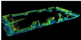
Fusing data sets from multiple sensors is a demanding requirements being seen more and more frequently in client specifications, typically combining photogrammetry or laser data with multibeam sonar data to create a seamless image of structures above and below the waterline. RESON have now prepared the PDS2000 software package to combine data under the waterline with data above the waterline to show breakwaters and harbour walls.
