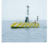
SEA-KIT's 12m Uncrewed Surface Vessel (USV) *Maxlimer* returned to Plymouth on Friday after 22 days of remote survey operations on Europe's continental margin. Since late July, the USV has mapped over 1,000sq km of ocean floor, controlled around the clock by SEA-KIT via satellite communications from its Remote Operation Centre in Essex. Notably, the uncrewed vessel returned to
